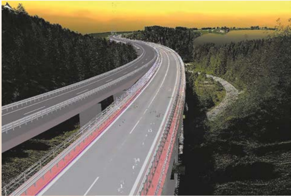
BIM pilot project: 2 nd Gauchach Valley Bridge: Existing conditions from a point cloud and designs.
